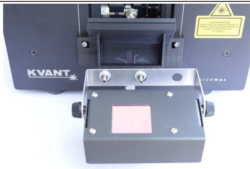
Fig. 1: Typical installation of the KB2D interactive device for a laser Harp application.
