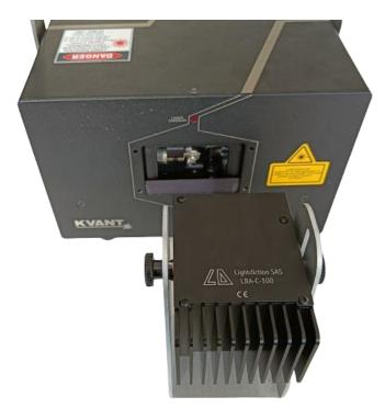
Start your "Lightdiction - Beam Analyzer" software. Select the LBA-C-100 sensor from the list, then start Streaming.
