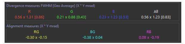
The LBA-C-100 is displaying the spot pattern as if it was projected at the "infinity". To align the RGB and B or stacks of diodes, we should see 1 single spot on the LBA-C-100, with all colors superimposed.
